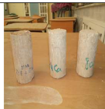
Figure .5. Tuff blocks reinforced with cardboard
