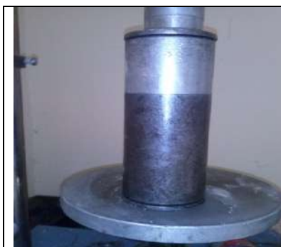
Figure .3 . Mould used for the manufacture of tuff blocks
