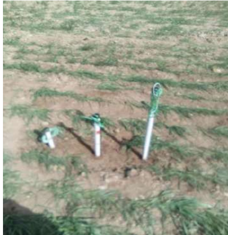
Figure 4. Tensiometers at different depths (0-20 cm/20-40cm and 40-60 cm)
